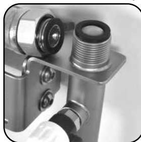
The safety sieve, included in the scope of delivery, prevents the resins from breaking out of the ion exchanger cartridge in case of any damage. Before installing the ball valve, place the safety strainer on the 3/4 "screw connection at the outlet of the connection fitting.
