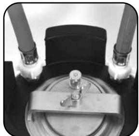
Loosen the screw connection.
