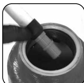
Filter nozzle must be present on the riser pipe.
